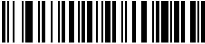
Interleaved 2 of 5 maximum length (0~50 bits)
